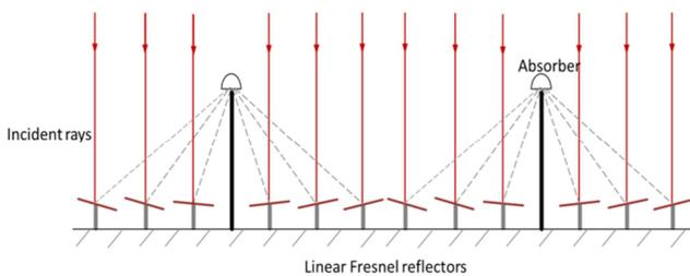
Figure 3. Linear Fresnel Reflector without interleaving of mirrors.
